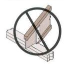
TJI® joist flange must bear fully on the plate. See detail BC on page 13.
