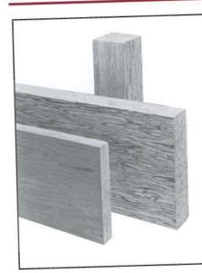
Microllam® laminated veneer lumber (LVL) is engineered with sheets of thin veneer structurally bonded together to make headers and beams which span much longer distances and support heavier loads than ordinary lumber. Microllam® LVL headers and beams are available in the following sizes:
