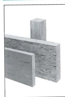
Microllam® laminated veneer lumber (LVL) is engineered with sheets of thin veneer structurally bonded together to make headers and beams which span much longer distances and support heavier loads than ordinary lumber. Microllam® LVL headers and beams are available in the following sizes:
