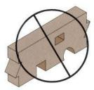
DO NOT cut, notch or drill holes in Microllam® LVL or Parallam® PSL except as indicated in chart and illustration.
