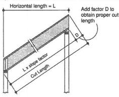
Actual cut length can be approximated by multiplying the horizontal length by the slope factor and adding the D factor.
